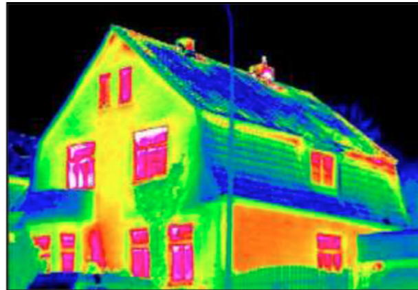
FIGURE XIV.1: INFRARED PHOTOGRAPH OF A HOME TAKEN IN WINTER. RED REPRESENTS WARM COMPONENTS, BLUE THE COLD COMPONENTS. / SOURCE: GOOGLE IMAGES
