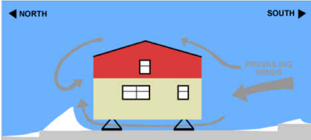
FIGURE 3.3: HOUSE AERODYNAMICS TO REDUCE SNOW ACCUMULATION SOURCE: CENTRE D'ÉTUDES NORDIQUES, UNIVERSITÉ LAVAL
