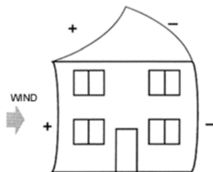
FIGURE VI.2: PRESSURE GENERATED ON A HOUSE BY WIND SOURCE: NRC ARTICLE: "UNE DÉFINITION DE PARE-AIR," PRODUCED AS PART OF BUILDING SCIENCE INSIGHT 86
