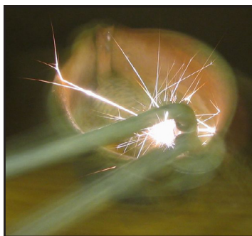
Figure 8.17.29 - Auer igniter in action
