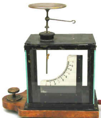
Figure 9.1.10 - Gold leaf electroscope
