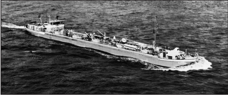
Figure 8.10.39 - The first tank vessel with entire hull from aluminum built in 1959
