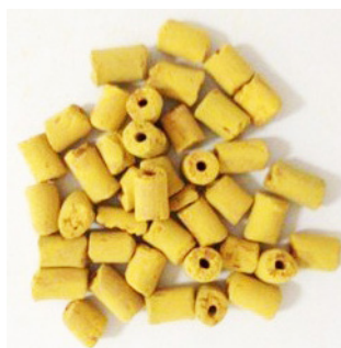
Figure 8.11.9 - Vanadium oxide catalyst for oxidation of SO_2
