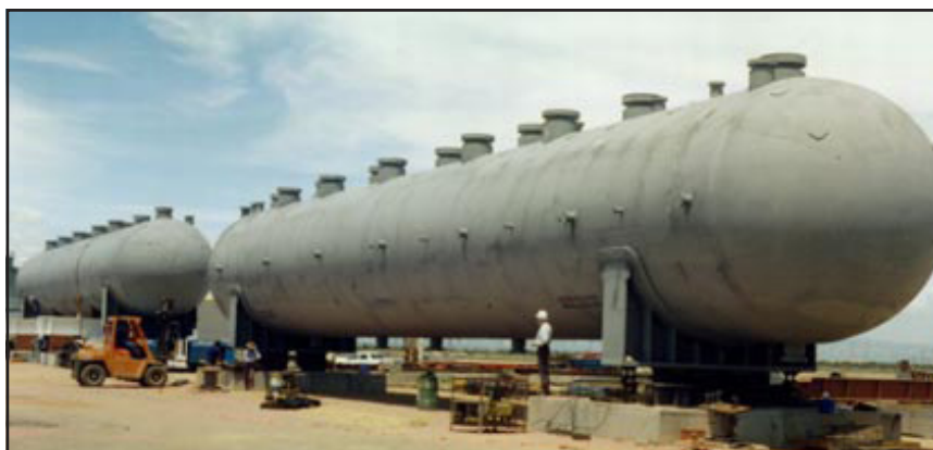
Figure 7.10.32 - Autoclave manufactured from titanium-clad steel
