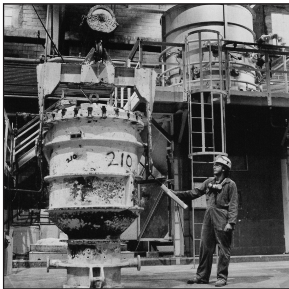
Figure 7.8.38 - Reactor containing a mixture of \text{UF}_4 and magnesium ready to enter the furnace for reduction to uranium metal
