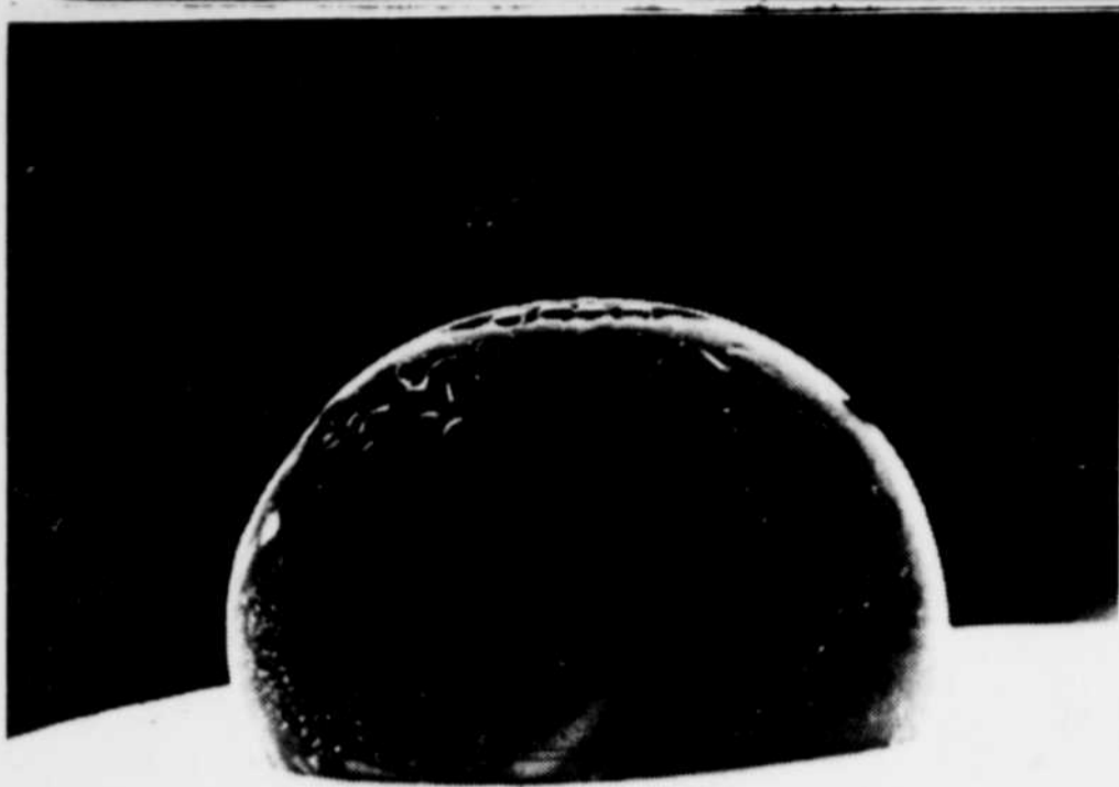
PLANET-LIKE protubance is not a new body in the firmament but a drop of tin on a silicon disc magnified some 40 times as photographed through a scanning electron microscope. Research into silicon crystal growth that could lead to higher efficiency solar cells is being carried out at Schenectady, N.Y., Research and Development Center of General Electric.
