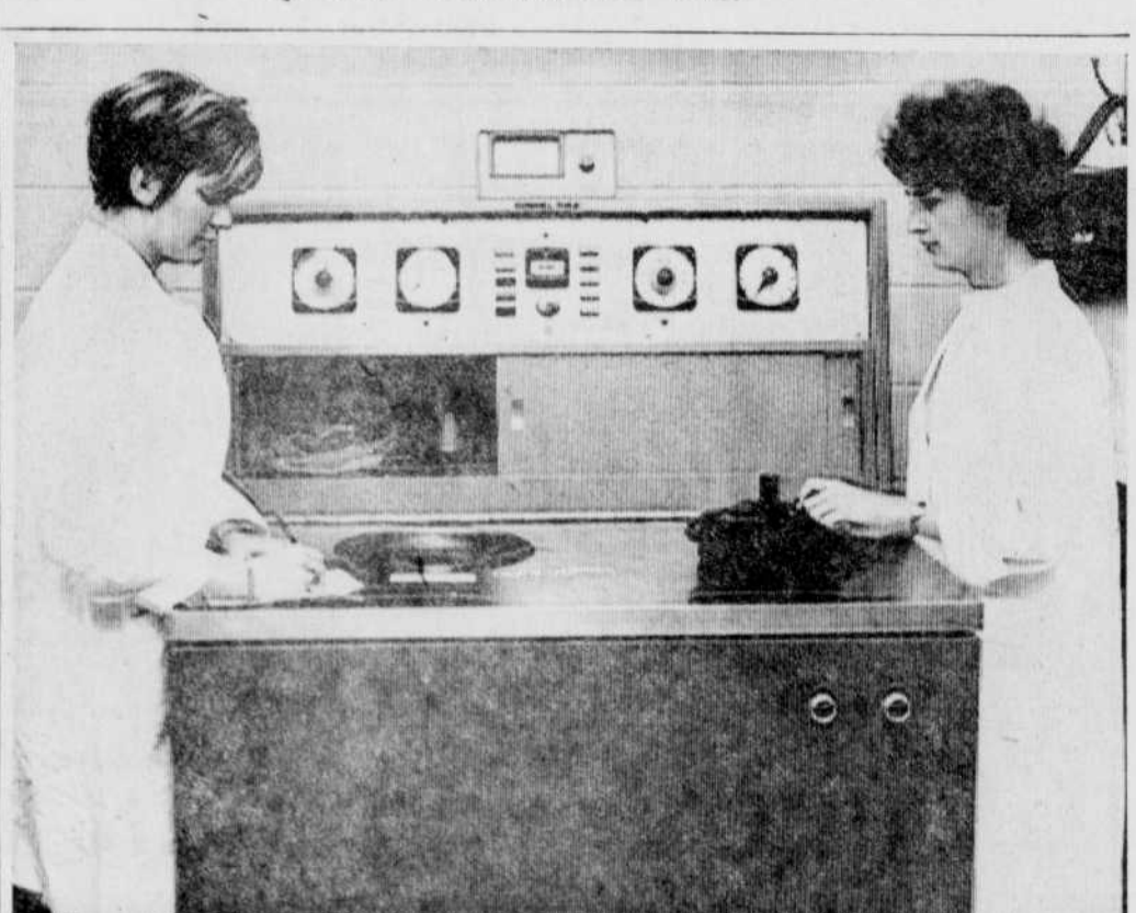
Miss Lyse Vanier (left) and Miss Monique Legars perform biological research with an ultracentrifuge. This instrument, used in biochemistry, separates various cellular fractions by speeds attaining a maximum of 60,000 R.P.M.
