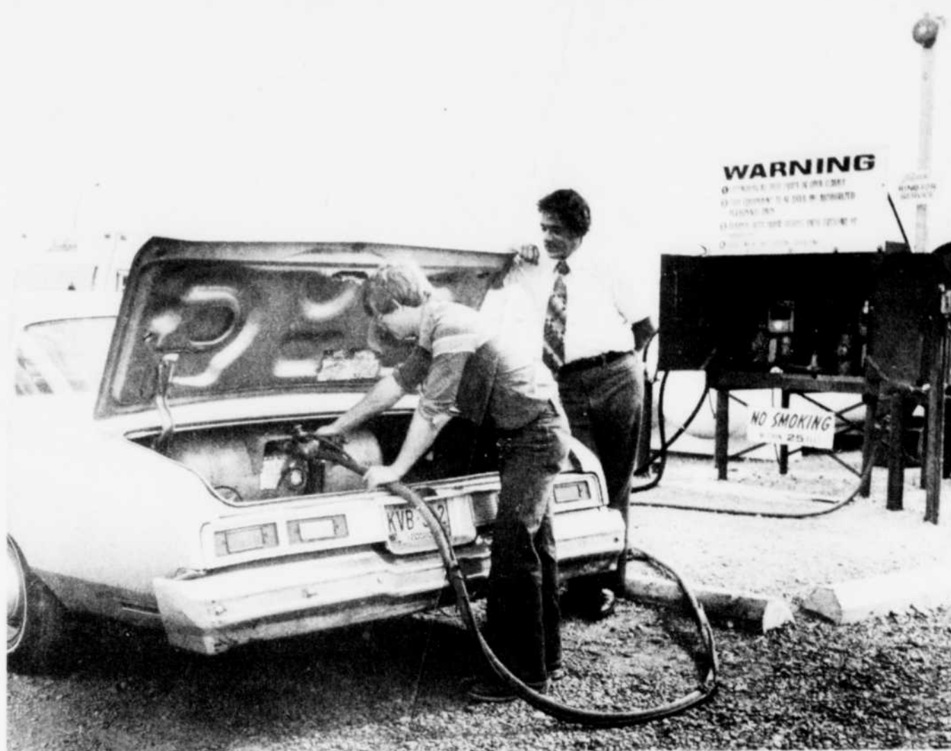
With the installation of a 22-gallon propane tank, this 1974 sedan has the option of using either liquefied propane gas (LP-gas) or regular gasoline at the flick of a switch.
