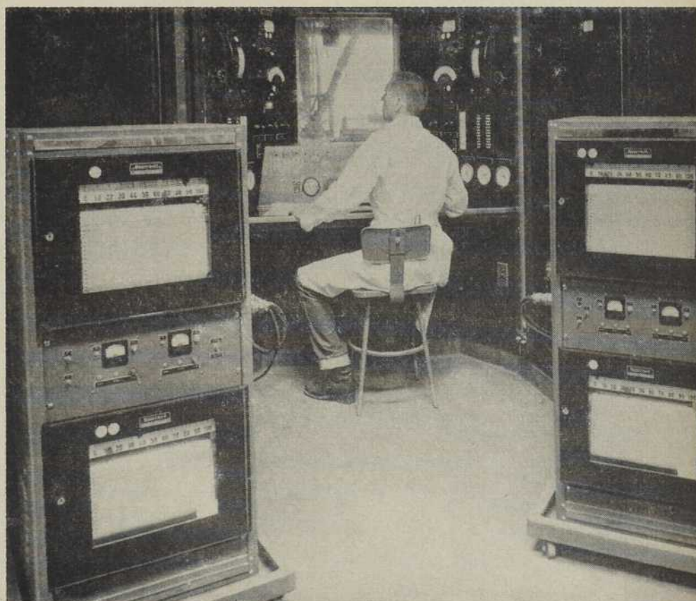
LAB TECHNICIAN VIEWS OPERATING GAS TURBINE THROUGH OBSERVATION WINDOW. RECORDS ON INSTRUMENTS IN FOREGROUND BECOME PART OF TURBINE'S PERMANENT FILE.
