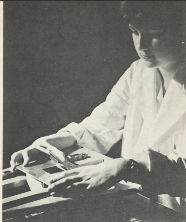
A laboratory assistant prepares photographic masks for semi-conductor devices and circuits by the step and repeat process.
