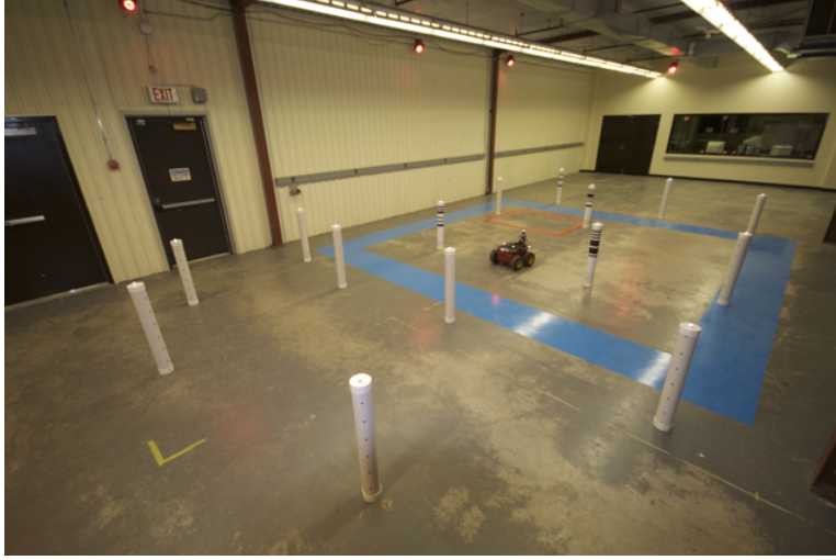
Figure 6: Experimental setup of the ‘Lost in the Woods’ dataset, courtesy of [13]. Truth measurements are obtained from a motion capture system.
