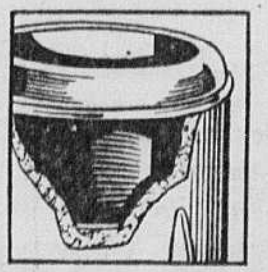
Cut-away view of a CONNOR-THERMO tub
