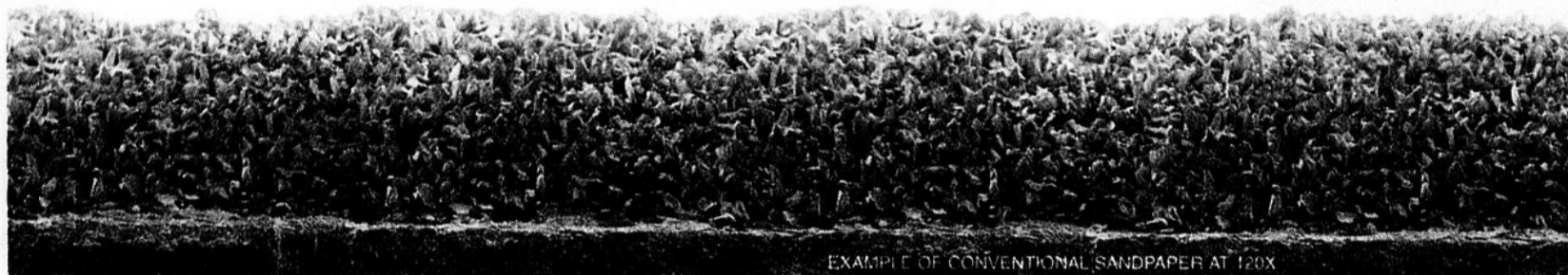
EXAMPLE OF CONVENTIONAL SANDPAPER AT 120X
