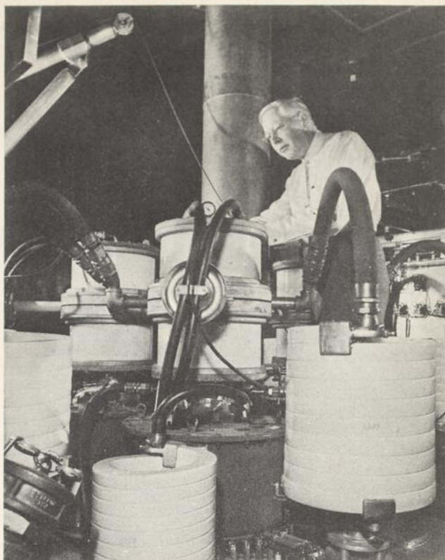
Array of RCA Superpower Tubes Provides Heat for "C" Stellarator Part of the largest electronic supply of its type ever built — an assembly of 6 to 10 superpower tubes, is shown here at Princeton University's "C" Stellarator fusion research facility, where the tubes are employed to start the heating of deuterium to ultra high temperatures. Here RCA engineer Nils Oman makes an adjustment on one of the 500 kilowatt super power tubes, which supply radio-frequency pulses to raise the deuterium in the stellarator to approximately one million degrees in an ohmic heating process.
