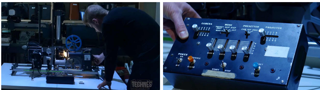
A JK optical printer, here used with a sequencer and a Bolex H16 camera; images taken from a demonstration given by filmmaker Philippe Léonard at Double Negative’s premises. See database entry.
