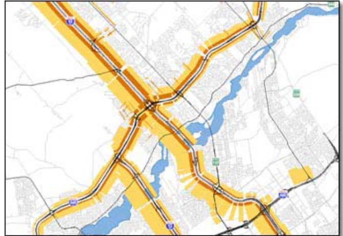
Proportion and origin of ramp users on the A-15 / A-640 interchange during morning rush hour (between 6 AM and 9 AM)
