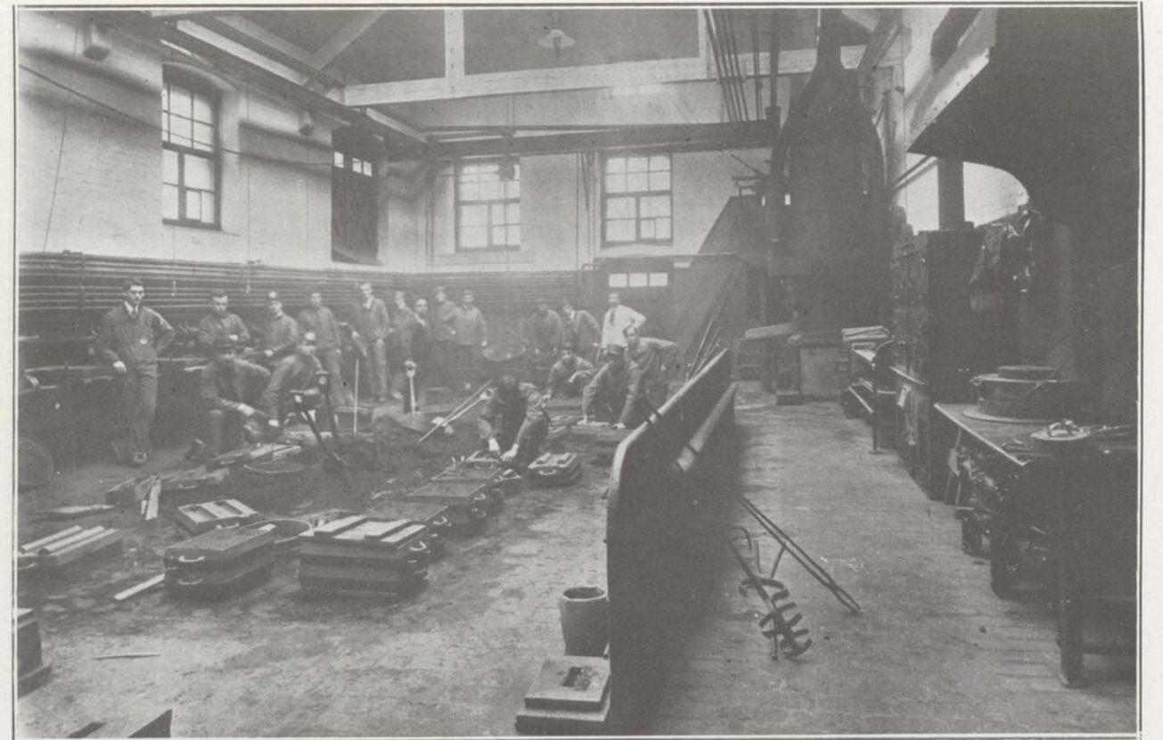
THE FOUNDRY.—This room has benches and apparatus for moulding and core-making. On the right a gas-fired brass melting-furnace is shown, and at the back a cupola for melting iron. A class of First Year students is shown at work.
