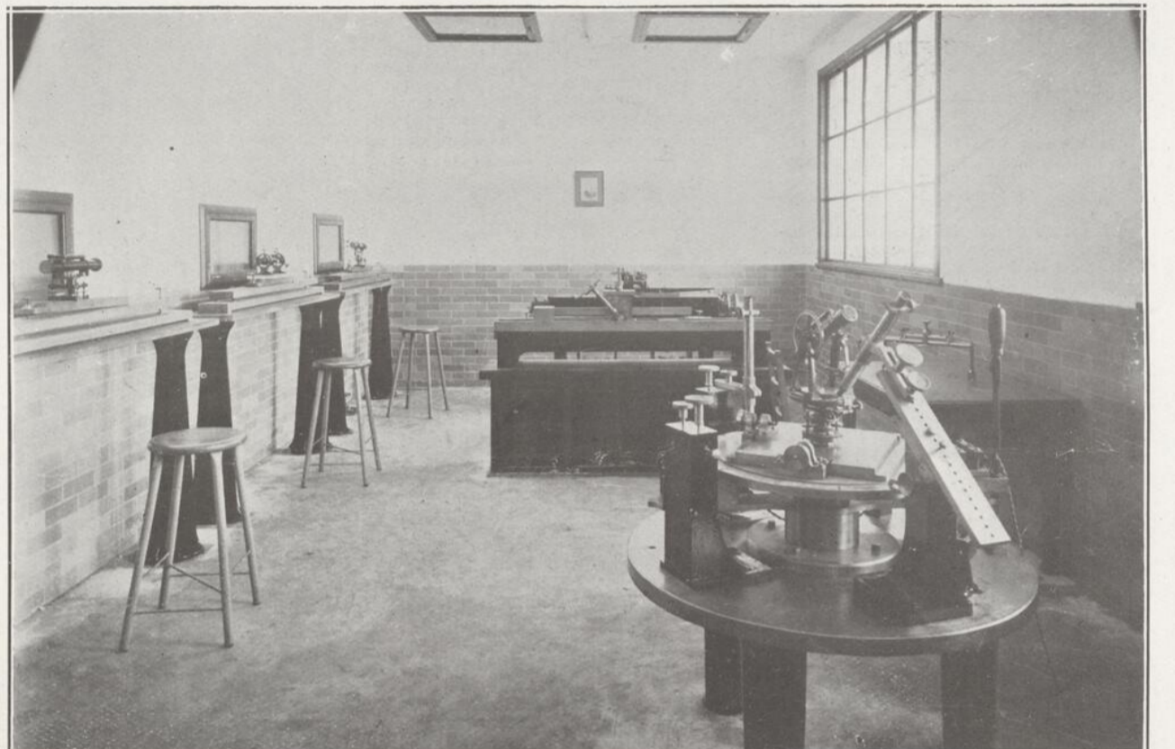
ONE OF THE GEODETIC LABORATORIES.—This room contains instruments for measuring the constants and determining the errors of surveying instruments. The instrument in the foreground is a circular comparator. This is one of the most important scientific laboratories at McGill.
