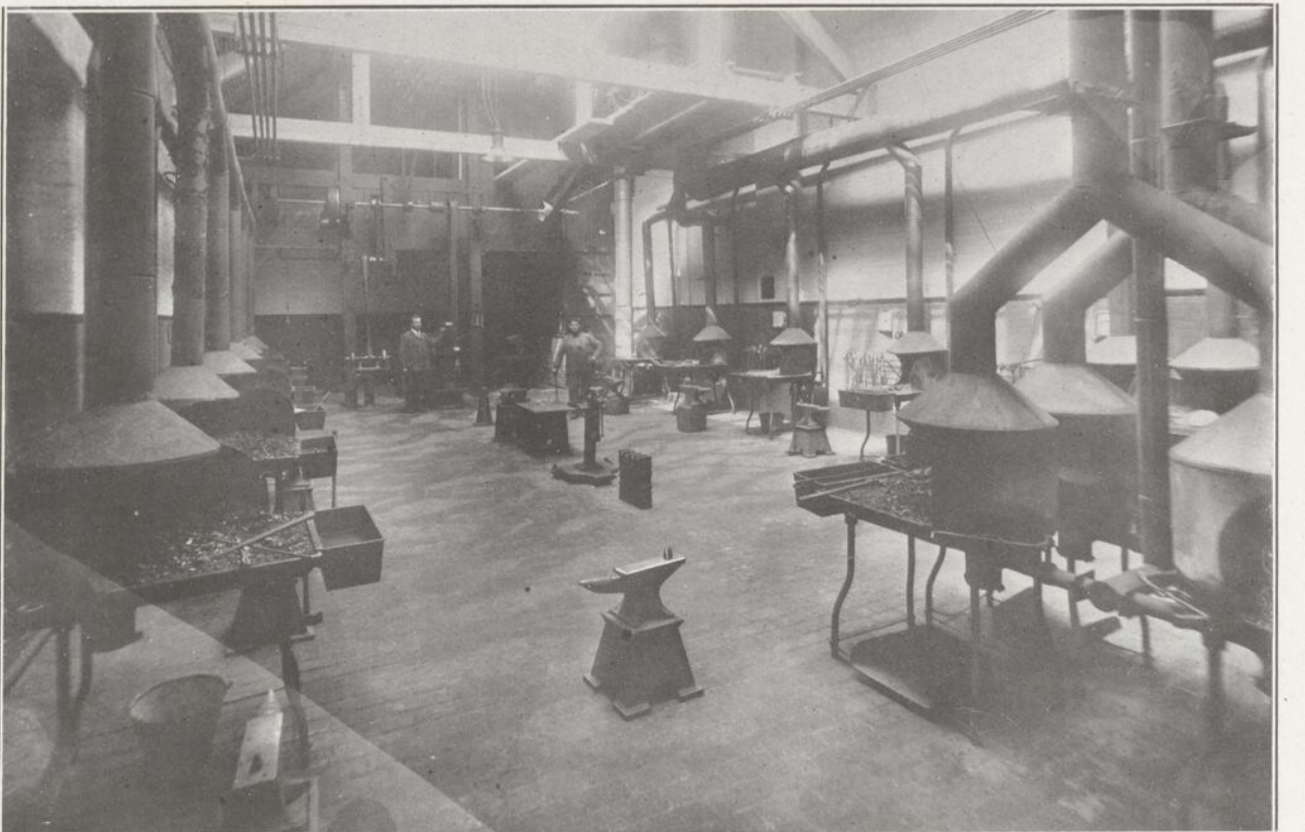
THE SMITH SHOP.—This room is provided with 16 Sturtevant forges, each power driven and connected with an exhaust-fan. There is a power-hammer and the necessary equipment of anvils and tools. (All photographs on this page by A. I. Rice, St. Catherine Street West.)
