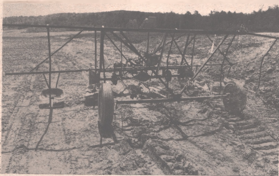
a machine towed along the rows on which 5 helpers sit and snip off strawberry flowers
