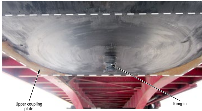
FIGURE 10 | Upper coupling plate and kingpin
