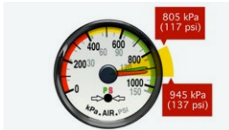
FIGURE 69 | Compressor stopping range
