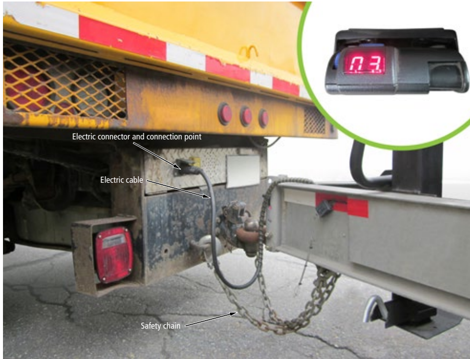
FIGURE 54 | Electric brake system FIGURE 55 (insert) | Electric brake intensity control
