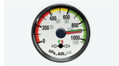
FIGURE 63 | Compressed air pressure gauge with two needles
