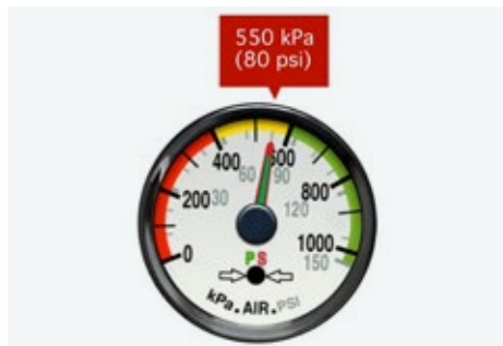
FIGURE 70 | Pressure gauge indicating a pressure of 550 kPa (80 psi)
