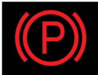
FIGURE 60 | Parking brake warning light
