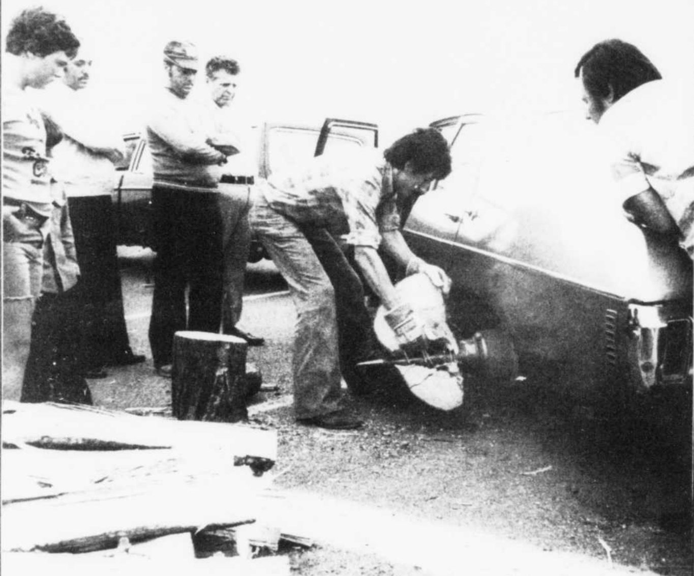
A revolutionary wood splitter has hit the market which contends you'll never use an axe again. Easily attached to either the power take-off on a tractor or to the wheel of a car, this new screw splitter will eclipse the existing machines now marketed.
