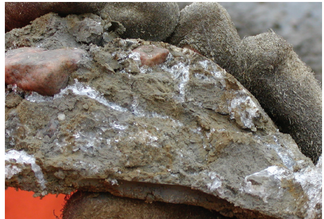
Ice lenses in this soil sample appear as white areas
