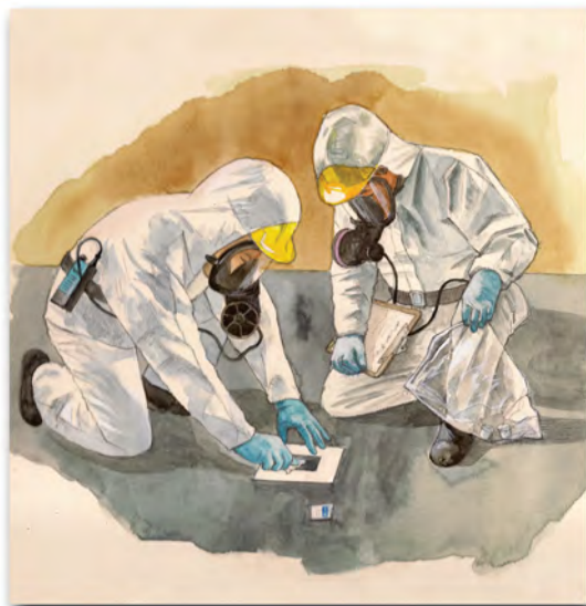
Figure 4: Wipe sampling with a moistened wipe
