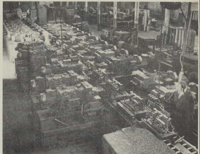
AUSTIN INLINE TRANSFER MACHINE OPERATING ON GEAR-BOX SHELLS FOR B. M. C. B SERIES 1½-LITRE POWER UNIT.
