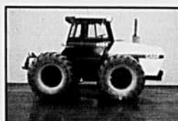
4694, 219 HP, roues doubles, 20.8-R38, 3 vitesses, power shift. St-Esprit
