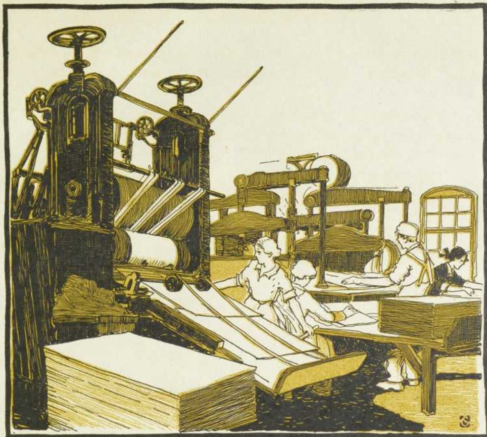
C A calender is shown on the left of this drawing and a plater on the right.
