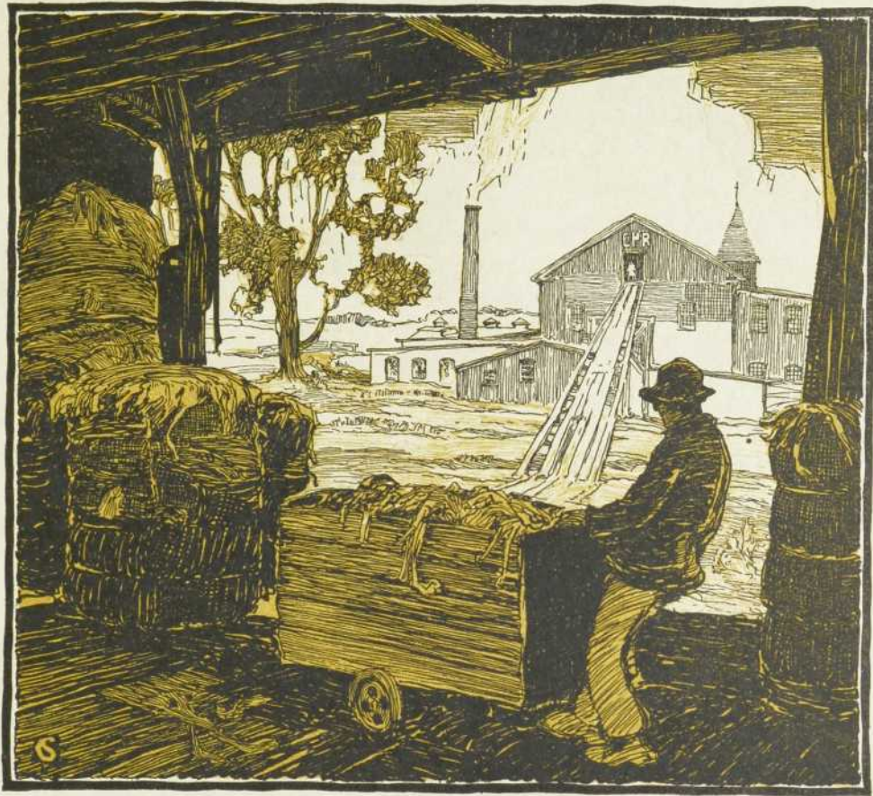
C The rags arrive in bales. They are elevated from the track-side shed shown in this drawing to the top of the mill in trucks drawn by cable.
