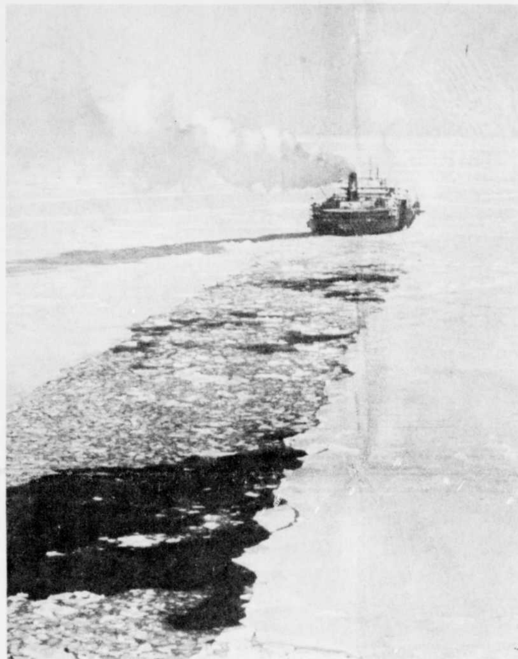
LOOKING FOR ICE — The United States supertanker Manhattan leaves a path of broken ice in its wake as it heads into the Northwest Passage. The tanker, on its second trip into the Arctic, is testing the feasibility of shipping oil from Alaska's North Slope to the eastern seaboard. (CP Photo)
