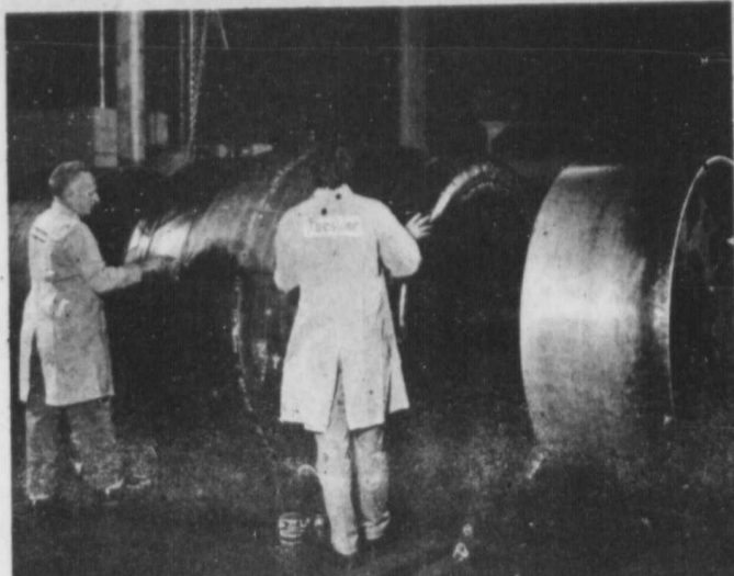
40 YEARS OF KNOW-HOW BUILDS AN $8,000 TIRE. With Forty years experience between them, this tire building team at Firestone's plant in Hamilton has what it takes to build Canada's biggest tire. The Super Rock Grip for giant earth-moving equipment stands almost nine feet high, weighs more than 2,700 pounds, and carries a price in excess of $8,000. Alfred Shepherd, on the left, is a craftsman with rubber and cord, with 33 years experience in Firestone's tire room. Compared to him Dave Gordon is a relative newcomer, with a seven-year record of service.
