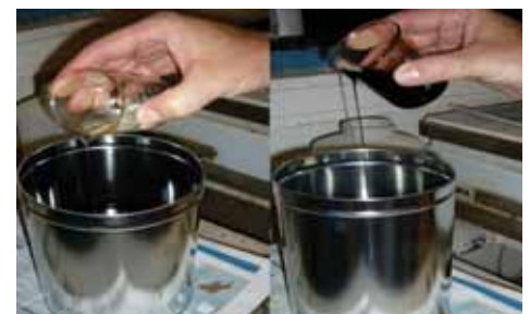
Photo 1. Additivation du liant lors d'une fabrication LEA® au CER d'Eiffage Travaux Publics // Binder modified with additives during the LEA® manufacturing process at the Eiffage Travaux Publics lab.
