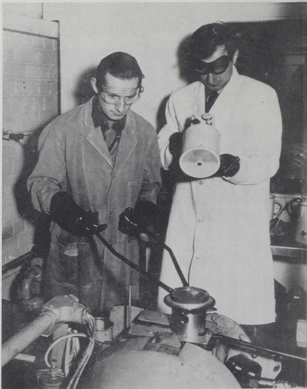
FIG. 1 — A RING IS FITTED WHILE ANOTHER PERSON IS MEASURING THE INTENSITY OF RADIATION TO WHICH THE OPERATOR IS EXPOSED.
