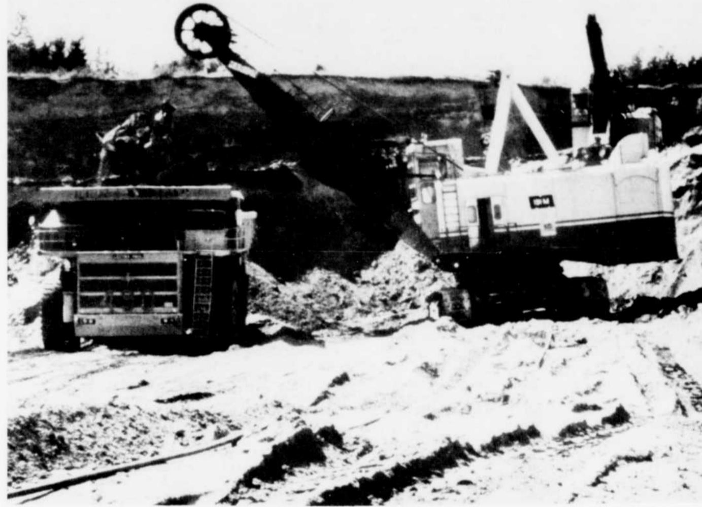
TRUCKS AND SHOVELS — Main mobile equipment in the open pit at the Johns-Manville mine includes 200-ton diesel-electric trucks; 100- and 120-ton diesel-electric trucks, 40-ton diesel trucks, electric shovels (4,160 volts) 6 to 15 cubic yards buckets and auxiliary equipment.
