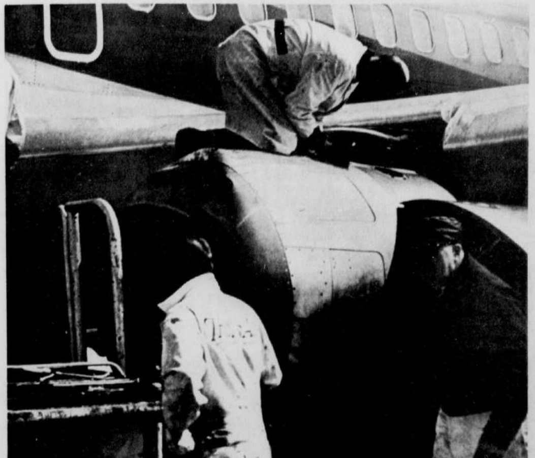
MID-AIR COLLISION — A dent in an engine housing of a Boeing 737 jet aircraft was
