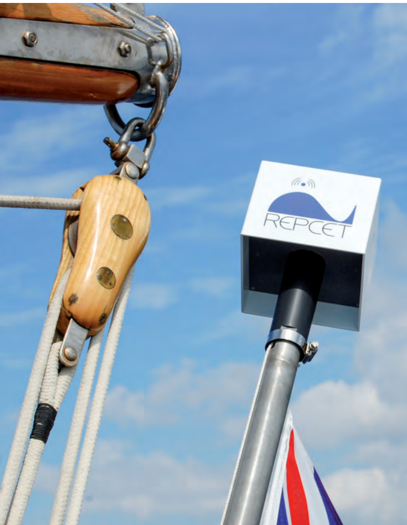
The REPCET ( repérage de cétacés en temps réel or real-time cetacean detection system) is a type of technology that allows for the real-time detection of whales in the Mediterranean Sea.
