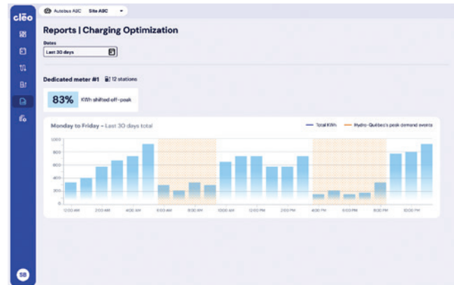
Example of shifting charging away from peak events on the Cleo smart platform.
