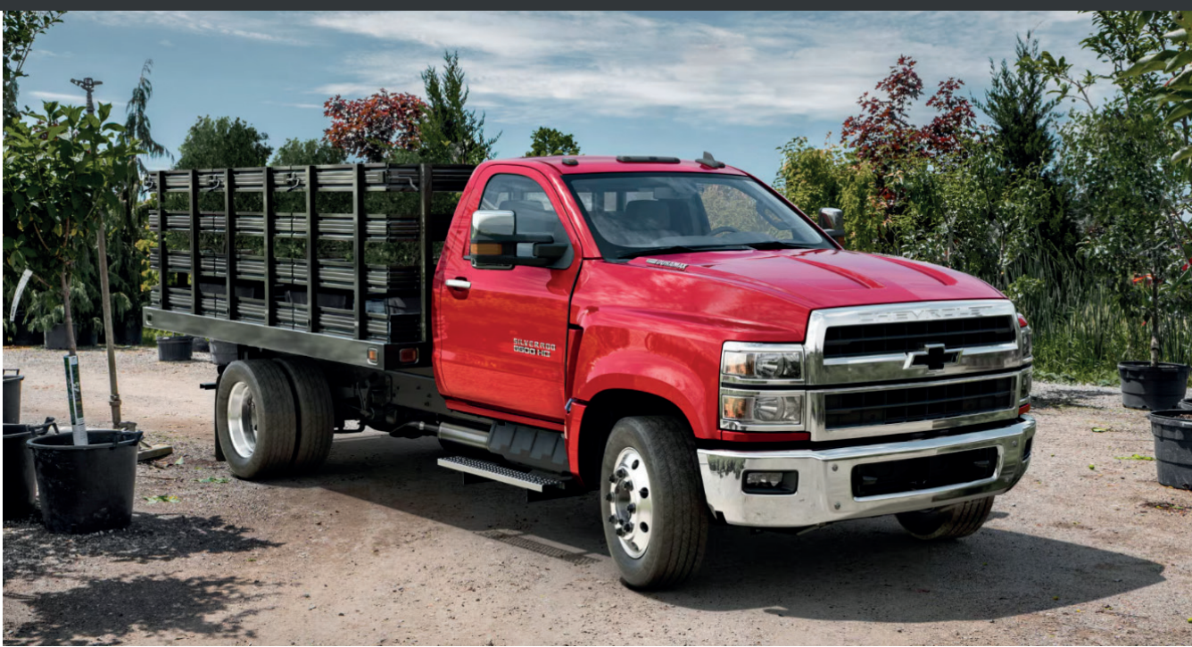
Flat frame rails maximize flexibility for upfitting use, for everything from stake beds to dump bodies.
