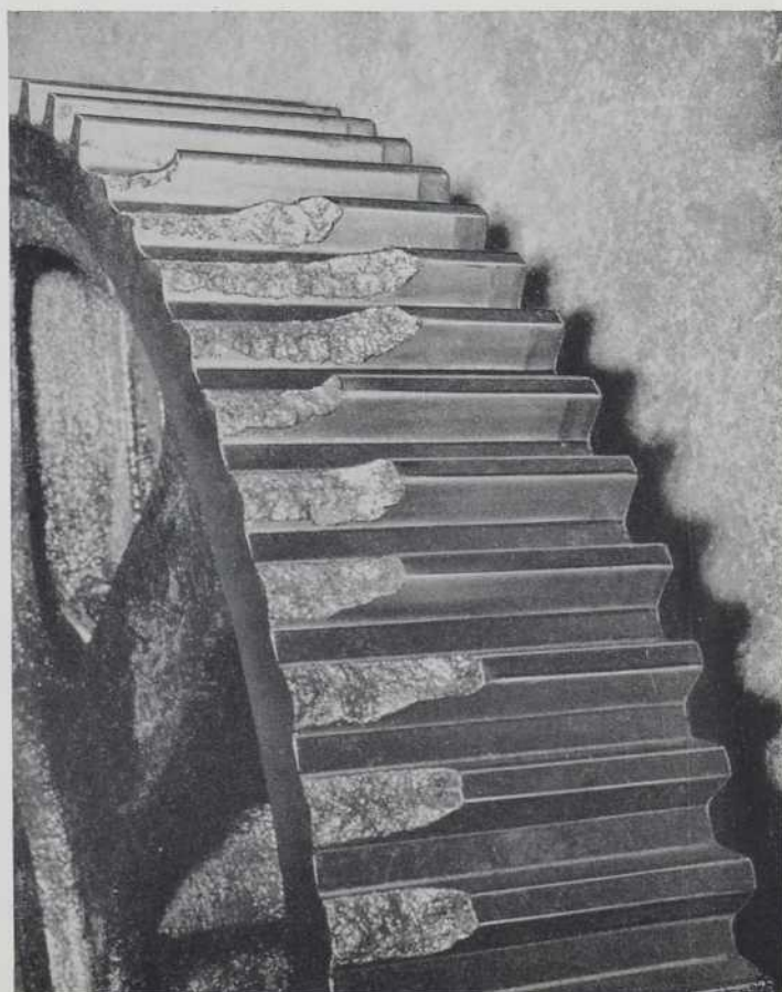
FIG. 14. — SPUR DRYER GEAR BROKEN DURING START-UP.
