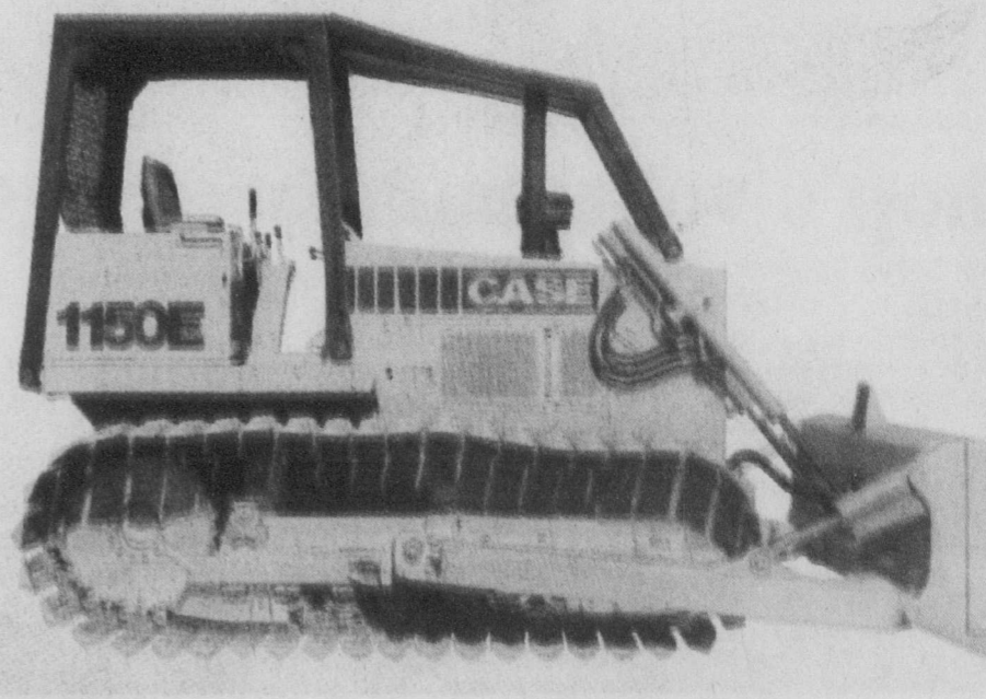
Model 1150E Case 113 net horsepower (84.3 KW) diesel Hydraulic angle/tilt/pitch blade to match job conditions LGP version offers less than 3.9 Psi (27 Kpa)
