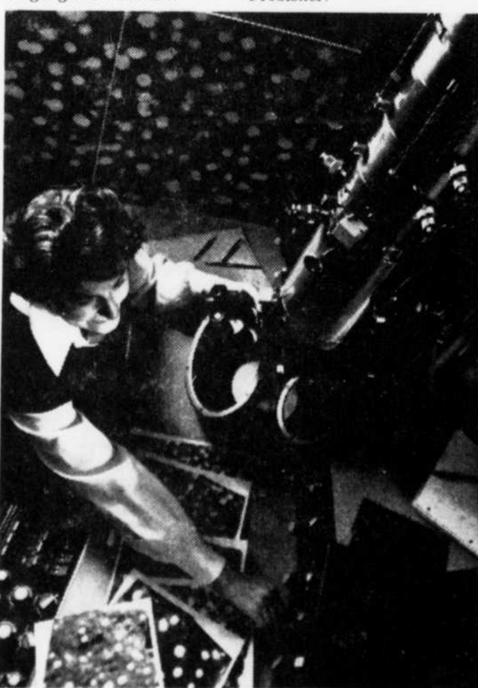
SWISS CHEESE appearance of magnified photos surrounding General Electric metallurgist Anna Turkalo at GE's research center in Schenectady, N.Y., is actually microscopic views of stainless steel samples bombarded with atomic particles before being installed in nuclear reactor plants. By blasting samples with radioactive material at speeds up to 2,500 miles per second, researchers are able to estimate the effect of a full year's exposure to atomic radiation thus sparing them extensive study before installation.
