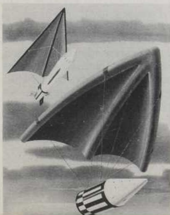
Another glider application is illustrated in artist's conception of these giant wings which are dropped from the prime mover in a folded position, and then automatically deployed in flight. Inflatable keel and leading edges are to be considered for this application.
