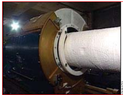
The future: Pipe-hugging asbestos removing robot
