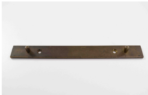
Raoul Barré's peg bar, which stabilizes drawings on the draughtsperson's work table.
