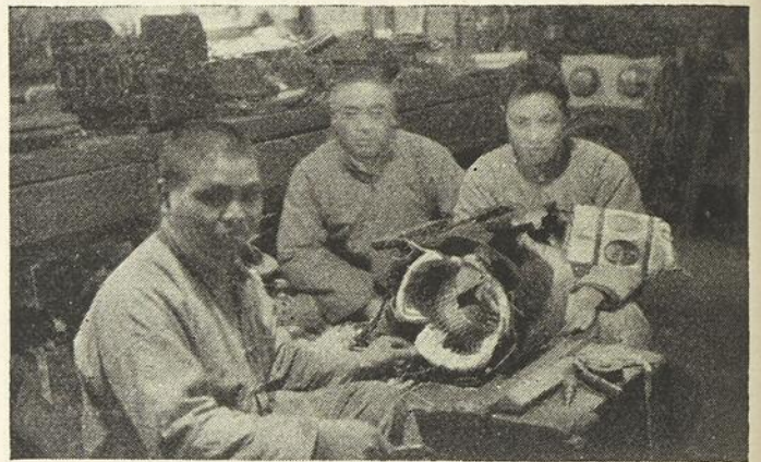
FIG. 4.—Chinese winders, rewinding electric motor in the electric shop of the new Engineering & Shipbuilding Co. Ltd.
