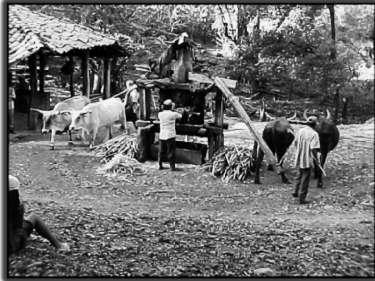
The trapiche, extracting juice from sugar cane on the farm La Caldera
