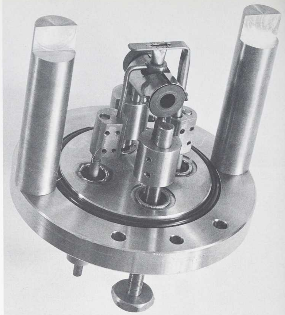
PHOTOGRAPH OF AN ACTUAL GRAPHITE OVEN USED IN EXPERIMENTS AT THE FOSTER RADIATION LABORATORY, MCGILL UNIVERSITY, CIRCA 1977.
