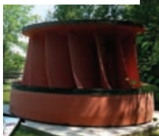
Turbine avant restauration. ▶
