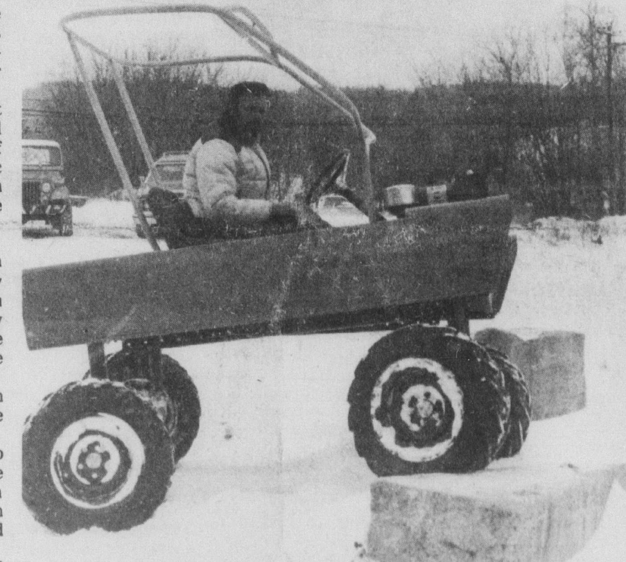
The incredible Quadractor can literally climb the walls because of its revolutionary design which features four-wheel independent drive.
