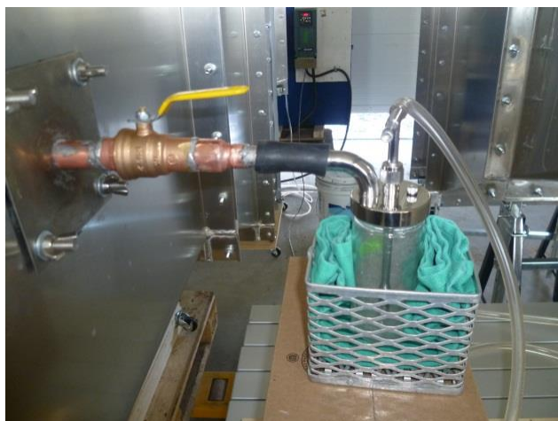
Figure 3 Experimental device for nebulizing viral aerosols
