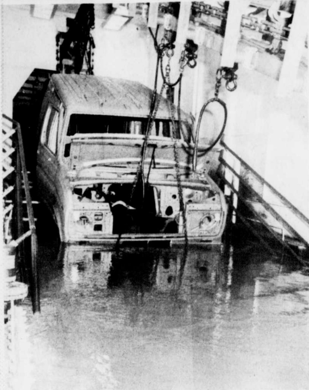
A BIG DIP — Ford of Canada has launched a new corrosion protection process in all three of its assembly plants for 1978-model production. Included is this improved electrocoat paint system. Here a 1978 Ford van body, being produced for the first time at the Oakville Assembly Plant, is submerged in a 105,000-imperial-gallon tank filled with electrically-charged primer paint. The new cathodic electrocoating system requires less electricity to cover greater areas and is especially suitable for applying protective primer to hard-to-reach nooks and crannies found in car, van and truck bodies.
