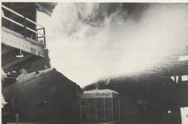
V.L.N. converter at Margam Works of the Steel Company of Wales uses large quantities of oxygen blown at bottom section.
