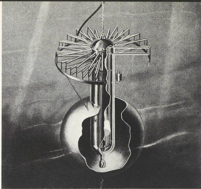
Power in the Deep —Undersea atomic plant will be developed by General Dynamics Corp., San Diego, Calif., as thermoelectric power source for naval units. Tubes at top change reactor heat to electricity.
