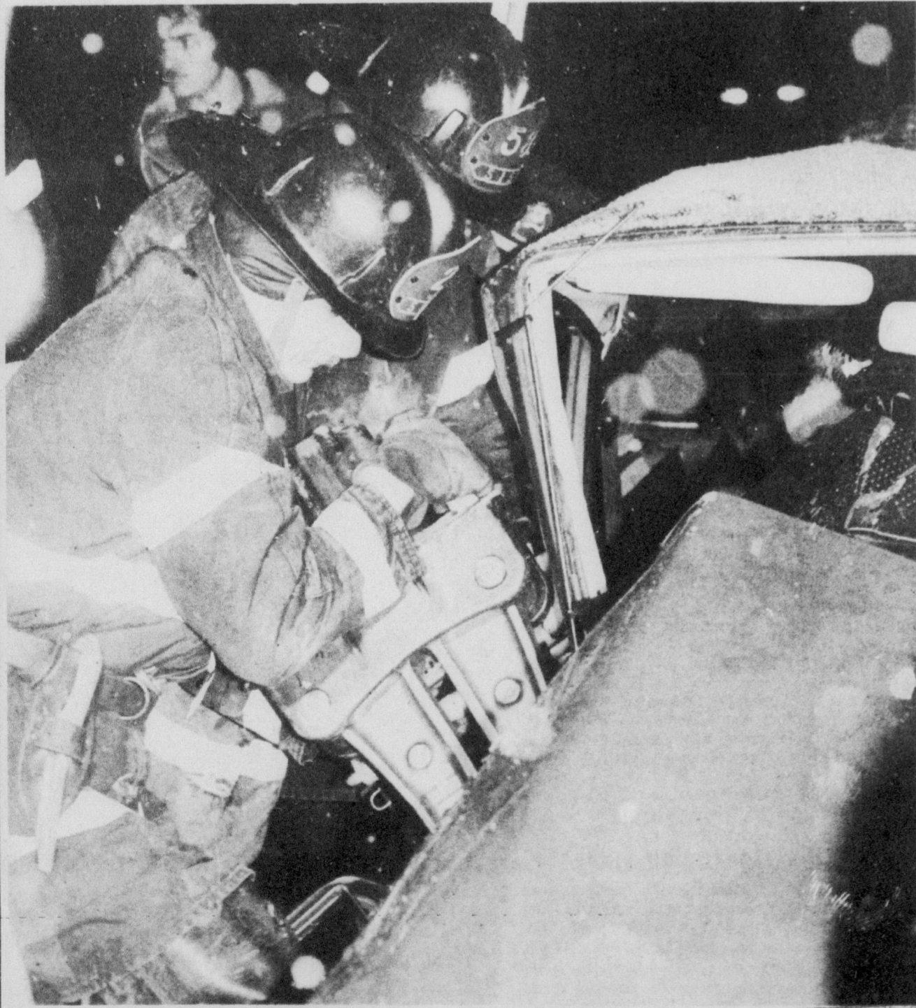
Lennoxville firefighters use their 'jaws of life' to cut apart the car to free a trapped passenger.
