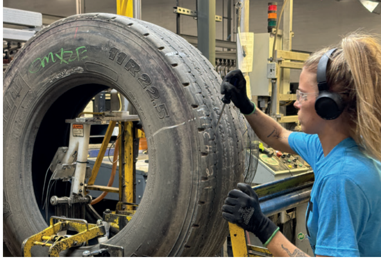
An operator removes stones from the tread.
