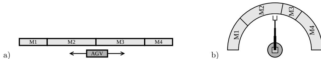
Figure 1: In a) an AGV transports parts between the machines moving in both directions along a straight line. In b) a material-handling industrial robot carries parts between the machines.
