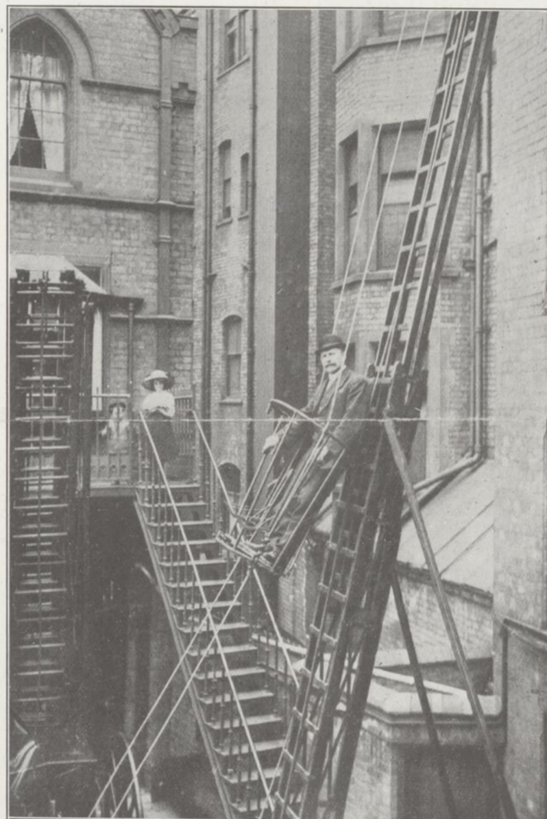
A NEW LIFE-SAVING APPARATUS—In Birmingham recently a demonstration took place of a new life-saving apparatus, consisting of a cradle for carrying persons from the upper stories of burning buildings to the pavements below. This apparatus is worked as follows: Cables are attached to the head of the fire escape, up and down which the cradle is drawn by means of a rope which passes through a pulley at the head of the escape. Attached to the cradle is an automatic brake, which immediately comes into action by the weight of the person if the hauling-rope should break. The cradle then at once becomes fixed on the guiding cables. The above picture shows the cradle as it would look if the hauling-line broke. (Copyright Topical.)
