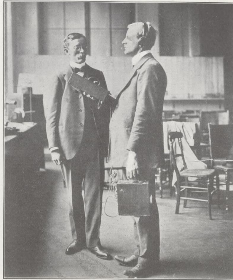
"EYES FOR THE BLIND"—A demonstration was recently given at the Science Museum at South Kensington of a new invention, by means of which light is made audible. The invention is based on the well-known properties possessed by selenium of changing its electrical resistance in proportion to the light which falls upon it. The above illustration shows a blind person tracing the course of a window by means of the invention. (Copyright Central News.)
