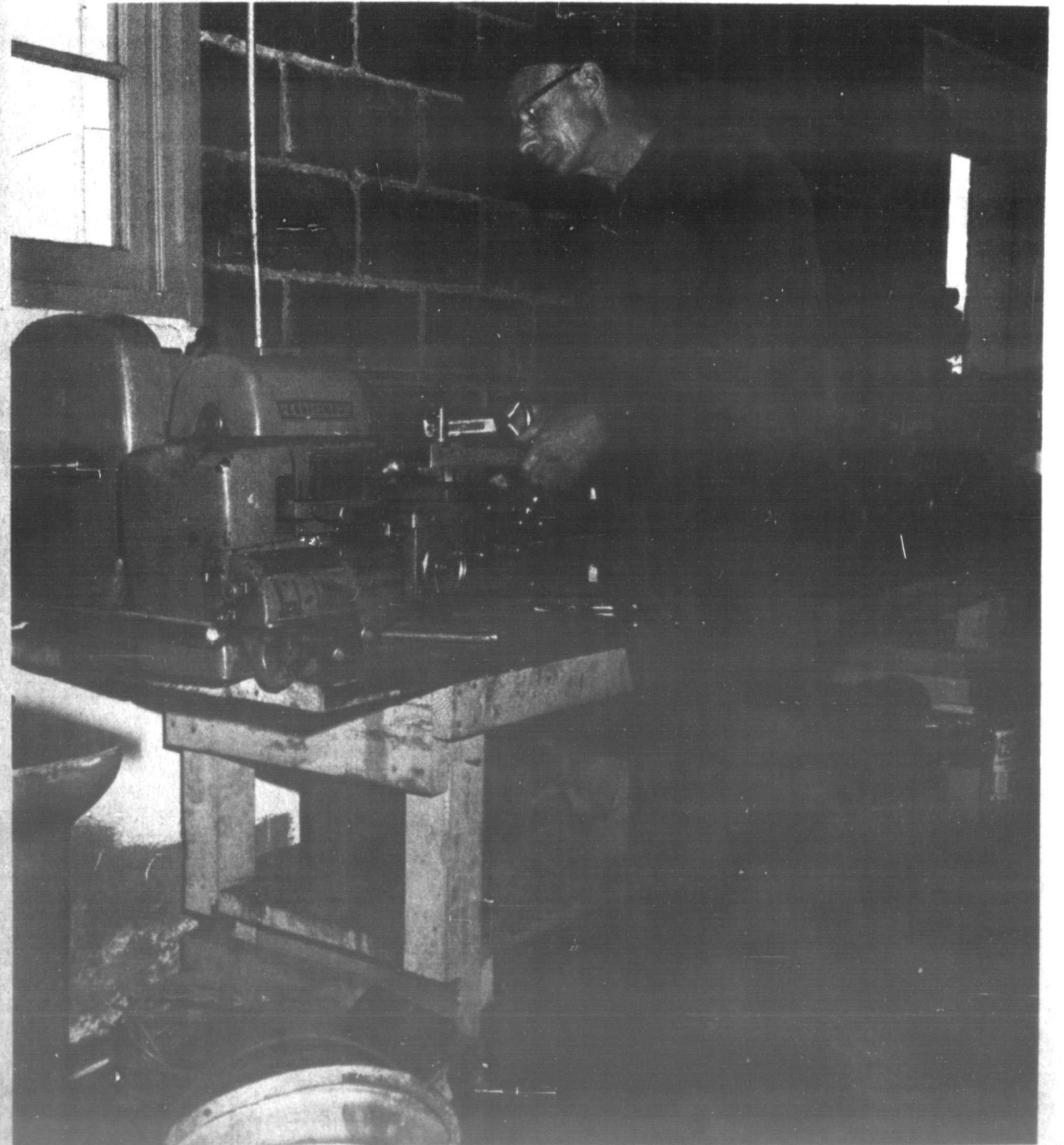
Stan Langdon making punches on the machine lathe.
