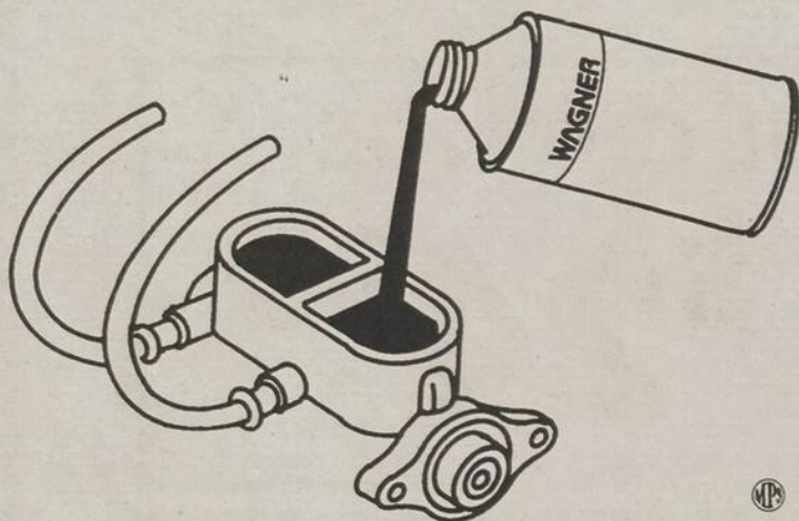
FILL THE MASTER CYLINDER to the full mark as noted on master cylinder reservoir or to 1/4 inch of the top with clean, fresh brake fluid. (Graphic courtesy of Wagner Brake Products)
